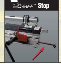
Allows Q-Cutter to remain installed on the track without interfering with bending. Simply slide Q-Cutter back to stop. Quick release allows for easy removal for transport.
